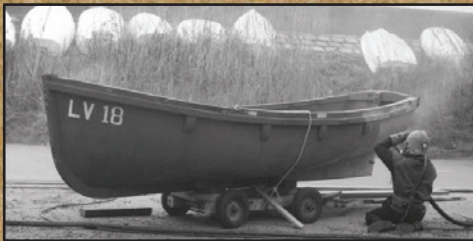
ORIGINAL LV18 BEING SAND BLASTED
